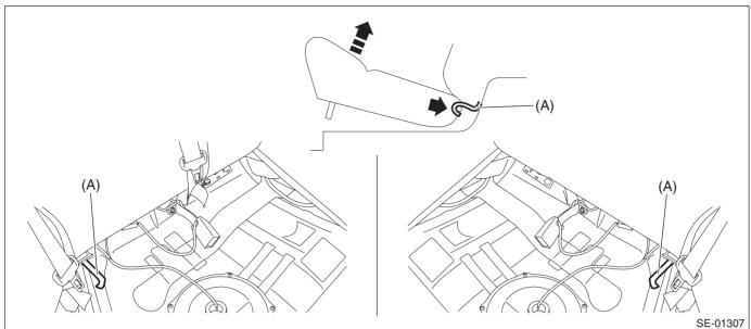
4) Release the clips and claws, and then remove the cover side sill - rear INN.
